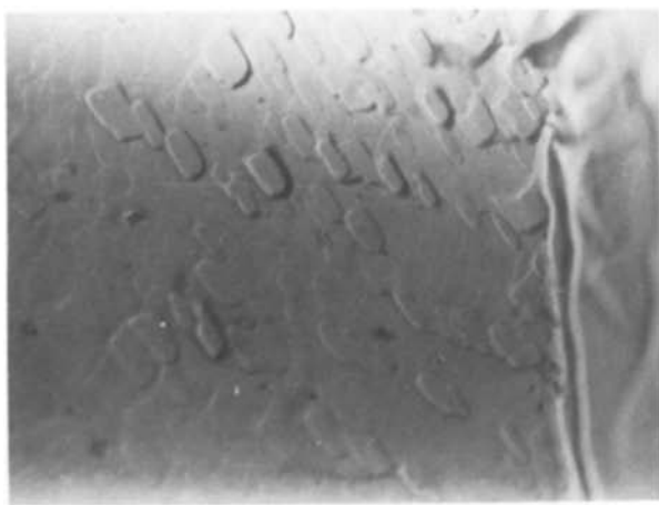
Figure 2 Brick-like elevations observed on (001) face (temperature difference 10° C) × 823.
